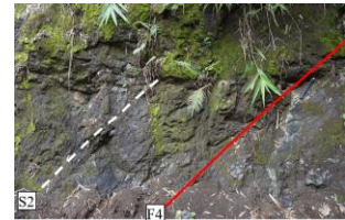
Photo 6. The characteristic of this deformation phase is the reverse, the left-lateral reverse fault system formation
